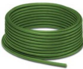
By the meter, Installation remote bus cable, INTERBUS, shielded, PUR, may green RAL 6017, 9-wire (3 x 2 x 0.22 mm<sup>2</sup> + 3 x 1 mm<sup>2</sup>), color single wire: green-yellow, white-brown, gray-pink, red, blue, green/yellow, fixed installation
